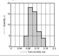
17-(2). Turn on time distribution (C type) Load voltage: 10V (DC) Continuous load current: 80mA (DC)
