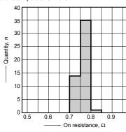
16-(2). On resistance distribution (C type) Measured portion: between terminals 3 and 4 Continuous load current: 80mA (DC) Ambient temperature: 25°C 77°F
