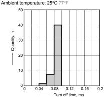
18-(2). Turn off time distribution (C type) Load voltage: 10V (DC)
