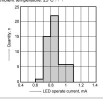
19-(2). LED operate current distribution (C type) Load voltage: 10V (DC)
